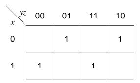
$$B=xy'z'+xyz+x'y'z+x'yz'=x \oplus y \oplus z$$
